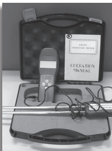
Figure 9. Moisture meter adapted for measuring moisture content of coffee
