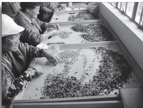
Figure 11. Sorting tables are used to facilitate the separation of defective GCB.
