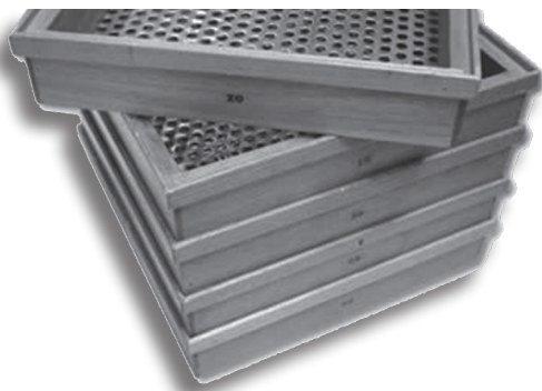
Figure 10. Set of sieves recommended for Arabica coffee.
